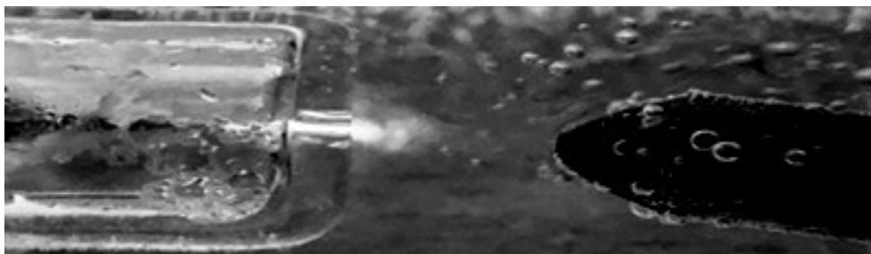
Fig. 3. Appearance of UDD in the cell (yellow-red glow was localised in the solution in the vicinity of the diaphragm)
