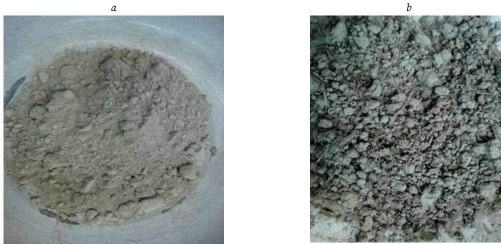
Fig. 1. Material samples: a – fly ash; b – ash with basalt fibres
